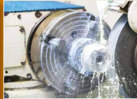
Get the performance of an oil soluble with the cleanliness of a synthetic! Tap Magic H<sub>2</sub>OX is formulated to provide excellent lubricity while eliminating the sticky messy film associated with heavy oil products. Designed for tool-dulling jobs like grinding, sawing, milling, boring, and reaming hard metals, Tap Magic H<sub>2</sub>OX can be used with any water-based metal cutting system to provide the following benefits:
